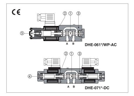
Spool type, two or three position direct operated valves with high performance threaded solenoids certified according the North American standard cURus.
